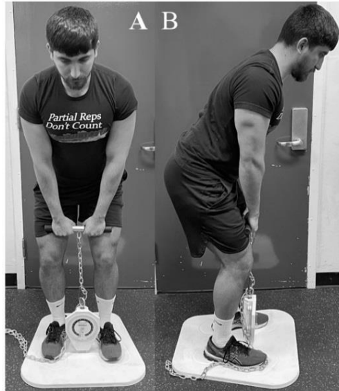
Figure 1. Frontal (A) and sagittal (B) view of the set-up for the leg/back dynamometer test.
